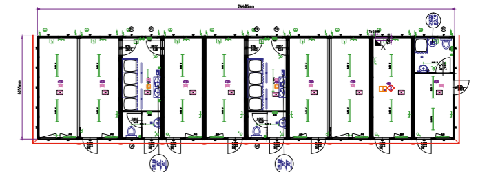
Changing rooms with sanitary facilities for two teams and referees
